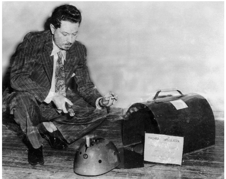
FIGURE 12.5 • William Grey Walter with one of his famous 'tortoise' robots photographed in 1951. He built two prototypes, Elmer and Elsie, in Bristol in 1948–9. Later six more were built, and displayed at the Festival of Britain in 1951. They had a photocell eye, two vacuum tube amplifiers that drove relays to control steering and drive motors, and a Perspex shell with a switch that operated when the shell contacted anything. They moved about autonomously in a lifelike manner, demonstrating the beginnings of artificial intelligence, and showed a form of self-preserving behaviour by crawling back into their charging hutch when their batteries ran low. In 1995 what was thought to be the last remaining Grey Walter tortoise was found and repaired by Owen Holland, and finally ended up in the Science Museum.
